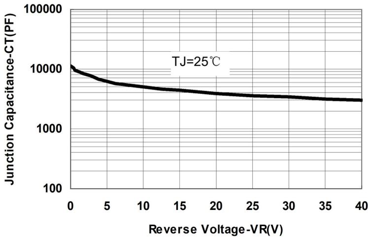
Fig.1-Typical Junction Capacitance
